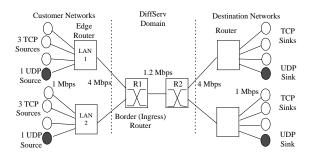
Fig. 4. Simulation network topology.
