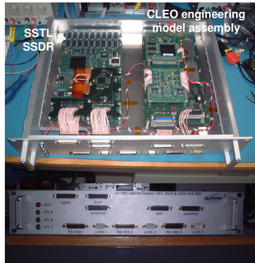
a. top view, before adding fans and heatsinks. b. front view of ports
