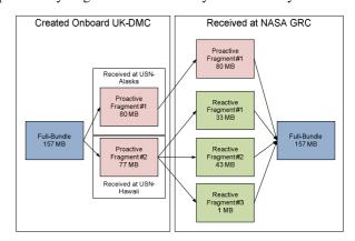
Figure 3 – Large File Transfers using Proactive and Reactive DTN
