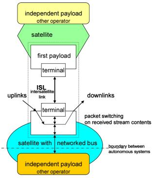
Figure 2: more advanced payload capable of sending stream, of switching on frames in received traffic, and of communicating with other payloads onboard.
