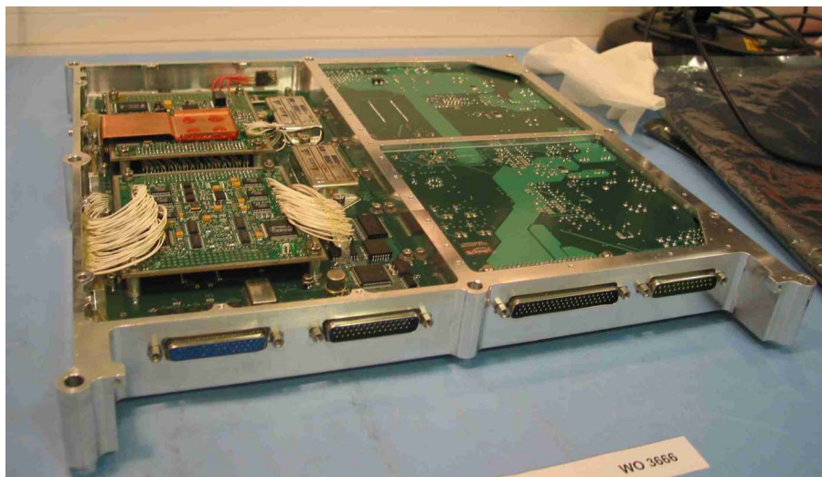
Figure 8.—Cisco router mounted in SSDL experiment tray.
