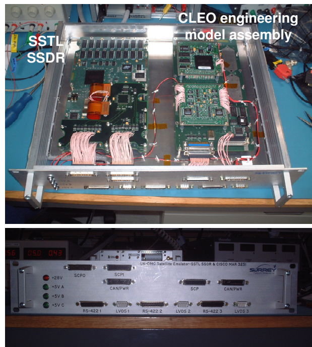
Fig. 2: CLEO ground-based configuration testbed – a. top view before addition of heatsinks/fans b. front view with interfaces and flexible patchbay.
