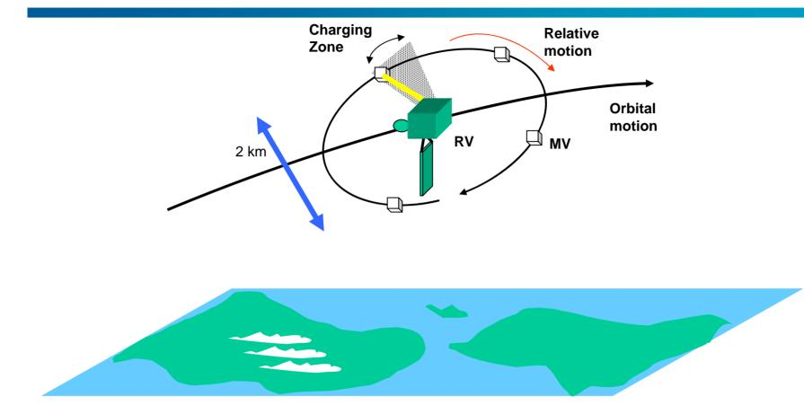
The RV would be in the center of the formation and distribute power to MV as they traverse a "charging zone"
