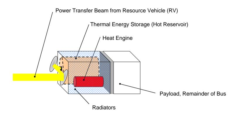
Within the MV the power transferred from the RV is absorbed as heat and then converted to electrical power by a heat engine for use by the payload and by the spacecraft bus
