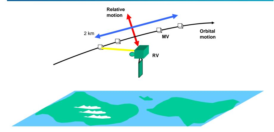
The MV are arranged in a linear formation in a common orbit and the RV is in an orbit with a significant wedge angle to this common orbit so that it comes into line-of-sight with each MV
