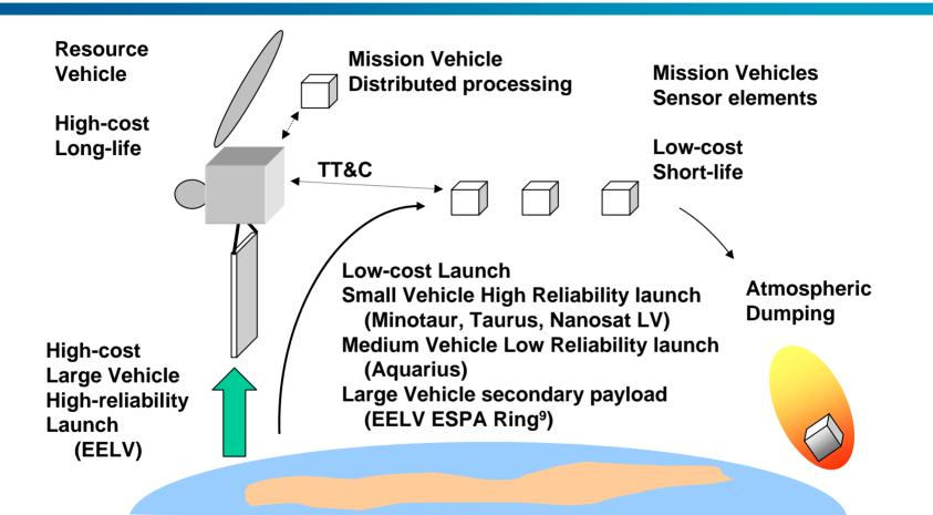
System architecture permits nearly continuous upgrade or reconfiguration of Mission Vehicle (MV) formation
