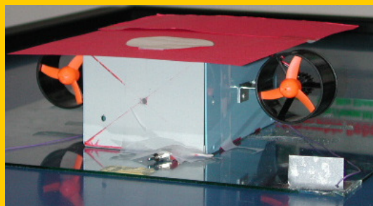
First cut with 2 fans for non-holonomic control
