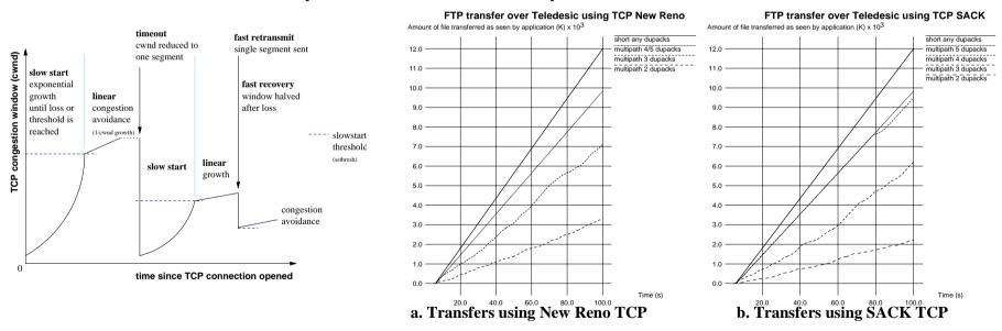
Progress of FTP transfer between terminals at Quito and Tokyo using Teledesic.
