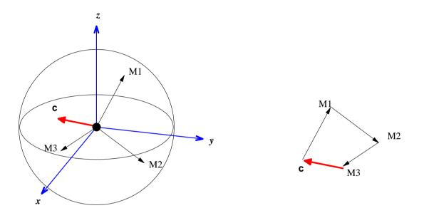
Satellites move, but terminals are fixed; place a fixed core using linear algebra (vector summation) and have its state inherited by the nearest satellite and passed on over time.
