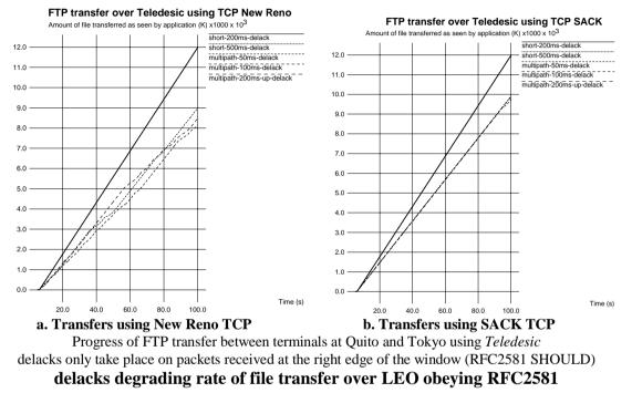
window faster in recovery than New Reno. This *should* increases flow performance - needed for multiple paths.
