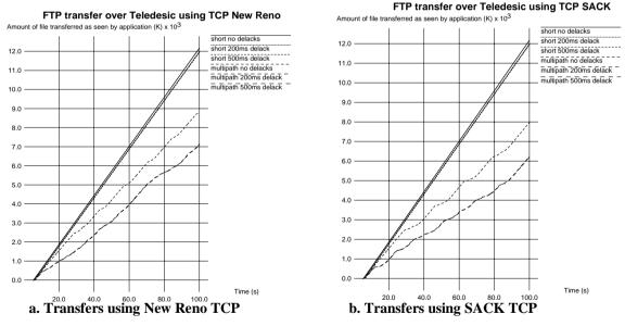
Progress of FTP transfer between terminals at Quito and Tokyo using *Teledesic*
