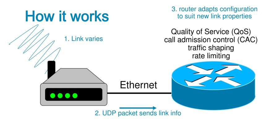
Modem sends UDP packet with information describing varying links to router when a link changes, and periodically.
