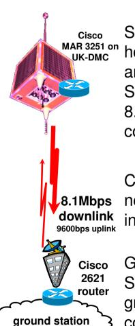
Satellite: each DMC satellite has multiple onboard computers. For housekeeping (the On Board Computer, OBC), for image capture and packetised transmission (the Solid State Data Recorders, SSDRs), for redundancy and survival. Interconnected by IP over 8.1Mbps serial links for data and slower CANbus for backup control; really a custom-built LAN.
